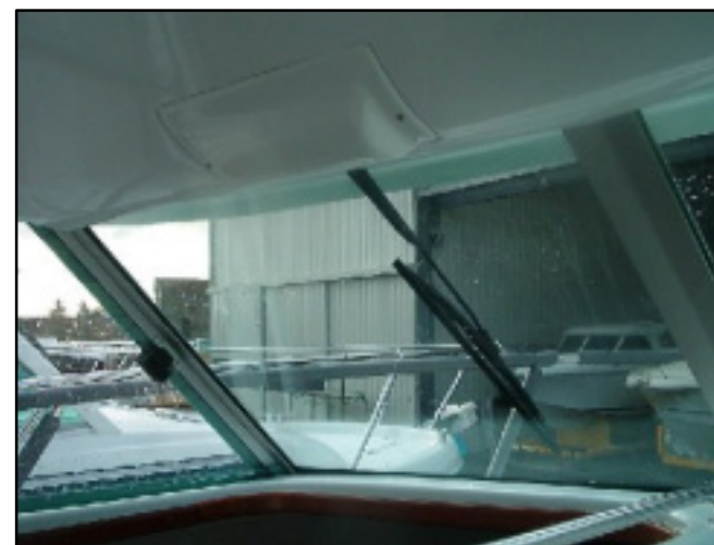
VUE DU 2° ESSUIE GLACE INTALLE Second windscreen wiper installed
