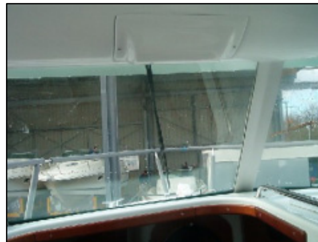
VUE DU 2° ESSUIE GLACE INTALLE Second windscreen wiper installed
